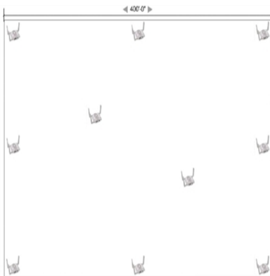
Figure 219: Rectangular Floor Plan AP Deployment
